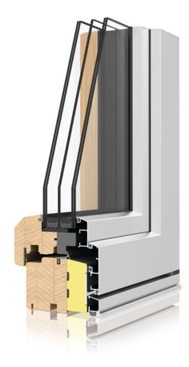
In uni\_one's Termoscudo system, a frame and sash of XPS are inserted between the wood and the aluminium, allowing extremely low thermal transmittance values to be achieved.
